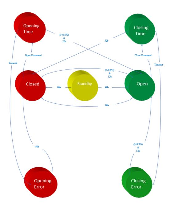
If **both circuit breaker contacts 52a and 52b** are available, they should be wired to the two physical inputs. These physical inputs are then assigned to the corresponding logical inputs: the circuit breaker 52a contact to the "52a Input" logical input, and the circuit breaker 52b contact to the "52b Input" logical input. The circuit breaker automaton is considered as having eight statuses: Startup, open, closed, error, opening time, opening error, closing time, and closing error.
