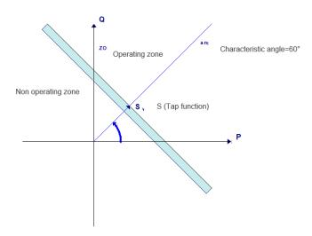
An operating zone is established based on the tap setting of the function and the setting of the characteristic angle. The function trips if the measured power is maintained in the operating zone for the time established using the corresponding time setting.
