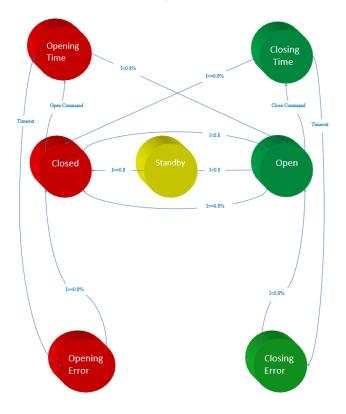
If only the circuit breaker **52a contact** is available, it should be wired to the corresponding physical input. This physical input is then assigned to the "52a Input" logical input. The 52b logical input is calculated internally as the negative of 52a. The circuit breaker performance is shown in the following finite state machine:
