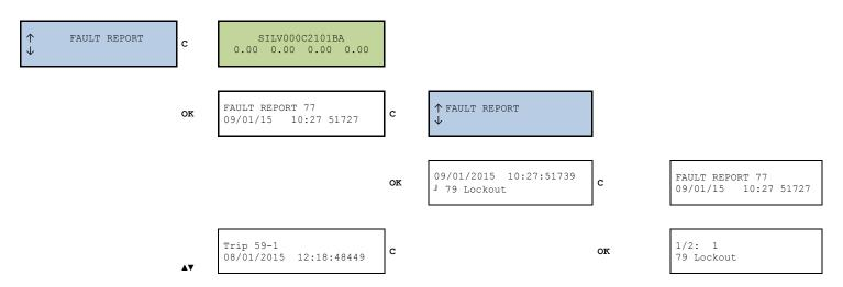
**NOTE**: if fault report is configured to a situation that does not cause trip screen then the fault report is identified with the number of report (example in the flowchart Fault report 77). If fault report is configured to a situation that originates a trip screen the fault report is identified with the trip (example in the Trip 59-1)
