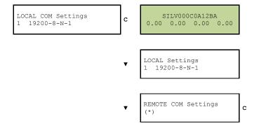
(\*) REMOTE COM parameters depend on model ( the used protocol can be IEC61850, DNP3.0, IEC60870-5-104, Modbus or IEC60870-5-103 depending on model)
