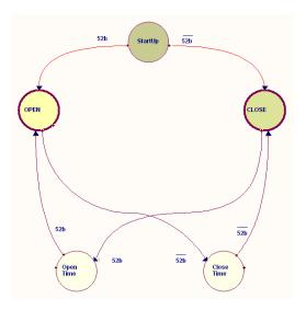
If both of the circuit breaker contacts 52a and 52b are available, they should be wired to the two physical inputs. These physical inputs are then assigned to the corresponding logical inputs: the circuit breaker 52a contact to the "52a Input" logical input, and the circuit breaker 52b contact to the "52b Input" logical input. The circuit breaker's automaton is considered as having eight statuses: Start, open, closed, error, opening time, opening fault, closing time and closing fault.
