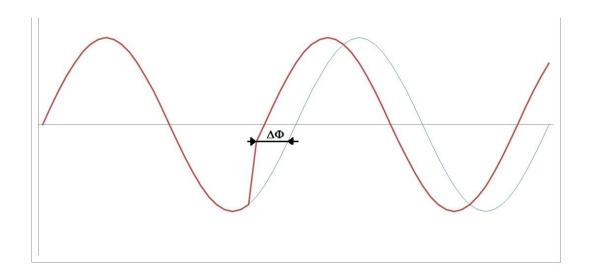
If  $\Delta \varphi$  exceeds the value adjusted in "level" setting, the function activates (trips) immediately. The accuracy is  $\pm\,5$  °.
