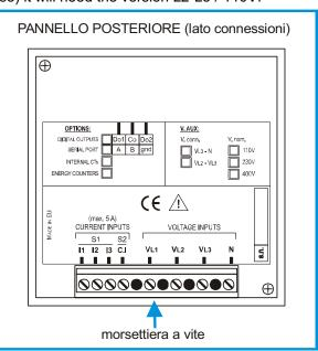
NOTE: It's a must to respect the phase sequence. The connections between current and voltage phase inputs must not be inverted (for example, CT placed on phase L1 must correspond to the I1 input). So as it is not correct to invert S1 and S2 terminals.
